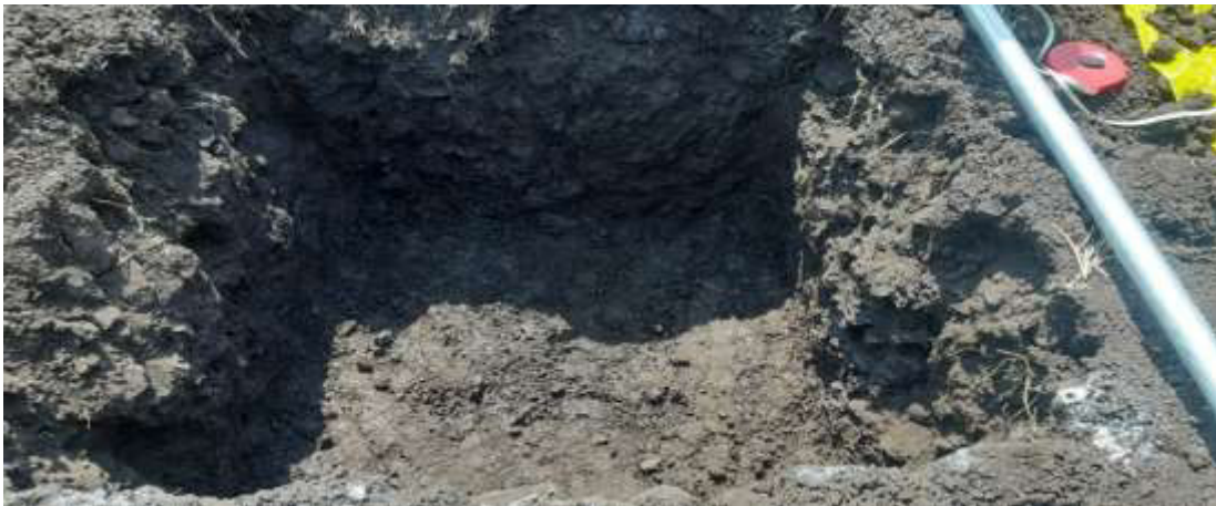
Plate 4. 1m × 1m pit from which soil was excavated layer wise to fill in inner tank of Lysimeter
