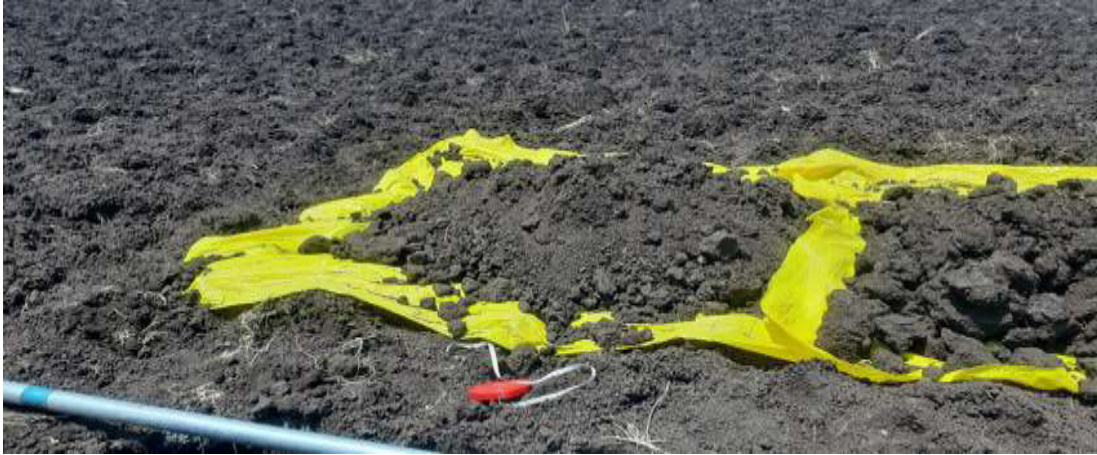
Plate 3. Layer wise heaves of soil
